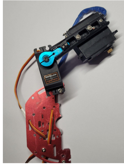
Figure 15. Metal body connected with elbow servo (own work)
